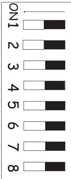
Do not program using the switches. All switches must remain in the off position. Acceptors come preprogrammed in order to work properly with the other electrical components of the machine. Use only the coupon to program the acceptor and only change sections 1 and 2.
