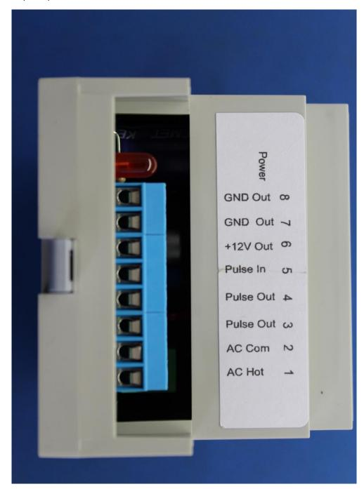
The diagram on the following page shows a typical installation with a Prowash manual bay timer, Microcoin QL coin mech and Nayax VPOS card terminal. Note that 24VAC COMMON is looped into one side of the output relay as the Prowash timer requires pulses of 24VAC COMMON to signal credit pulses on the coin input. Note that it may be necessary to loop 24VAC HOT, +12VDC or -12VDC through the output relay depending on the specific requirements of the timer being interfaced to.
