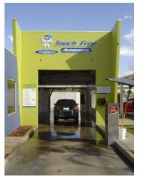
The Laserwash Touchfree Automatic offers a completely different service to your customers. Ensuring the Laserwash has a clear sign and height bar is essential. The height bar does not need to be positioned directly in front of the bay but must be located close by to prohibit large vehicles from entering and damaging your equipment.
